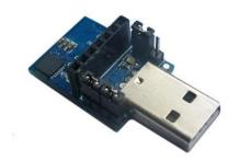
E30~E70 wireless module developed and produced by Chengdu Ebyte Electronic Technology Co., Ltd. is suitable for embedded application. Users usually connect it with MCU. The module has UART (TTL level) interface with its transparent transmission that makes it much easier for users to operate. To better simplify operation, the company has developed a USB to UART convert module E15-USB-T2.
